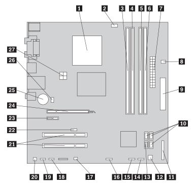
Figure 4. System board parts locations
